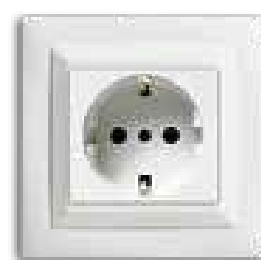
45DCB90T Prise Schuko standard Allemande 2P+T 16A 250V German Standard Schuko Socket 2P+T 16A 250V
